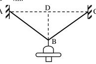
17. A bam AB of length 'l' is supported as drawn in the figure and subjected to equal but opposite vertical forces 'P' at two ends. Find the reaction at the supports 'C' and 'D'. [5]
